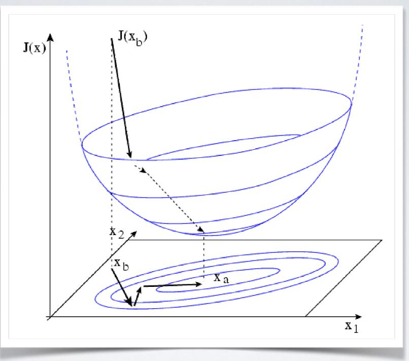
The minimization works by performing several line-searches to move the control variable to areas where the cost-function is smaller, usually by looking at the local slope (the gradient) of the cost-function.
