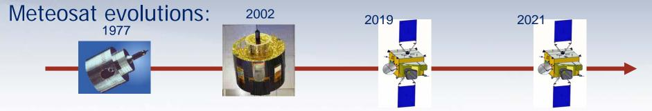
1 Imager – 3 Channels 2.25 km HR – 4.5 km 30 Min RC 1 Imager – 12 Channels 1km HRV – 3km 15 Min RC 1 Imager – 16 Channels 0.5 & 1km HR – 1 & 2 km 10 Min RC + LI
