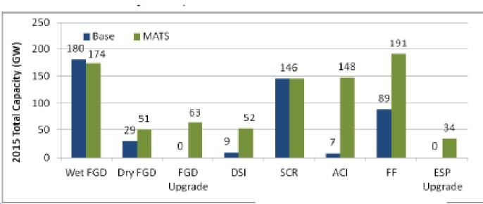
Retrofit pollution control installations on coal-fired capacity (by technology) with the base case and with the final MATS, 2015 (measured in GW capacity). Source: Integrated Planning Model run by EPA, 2011
